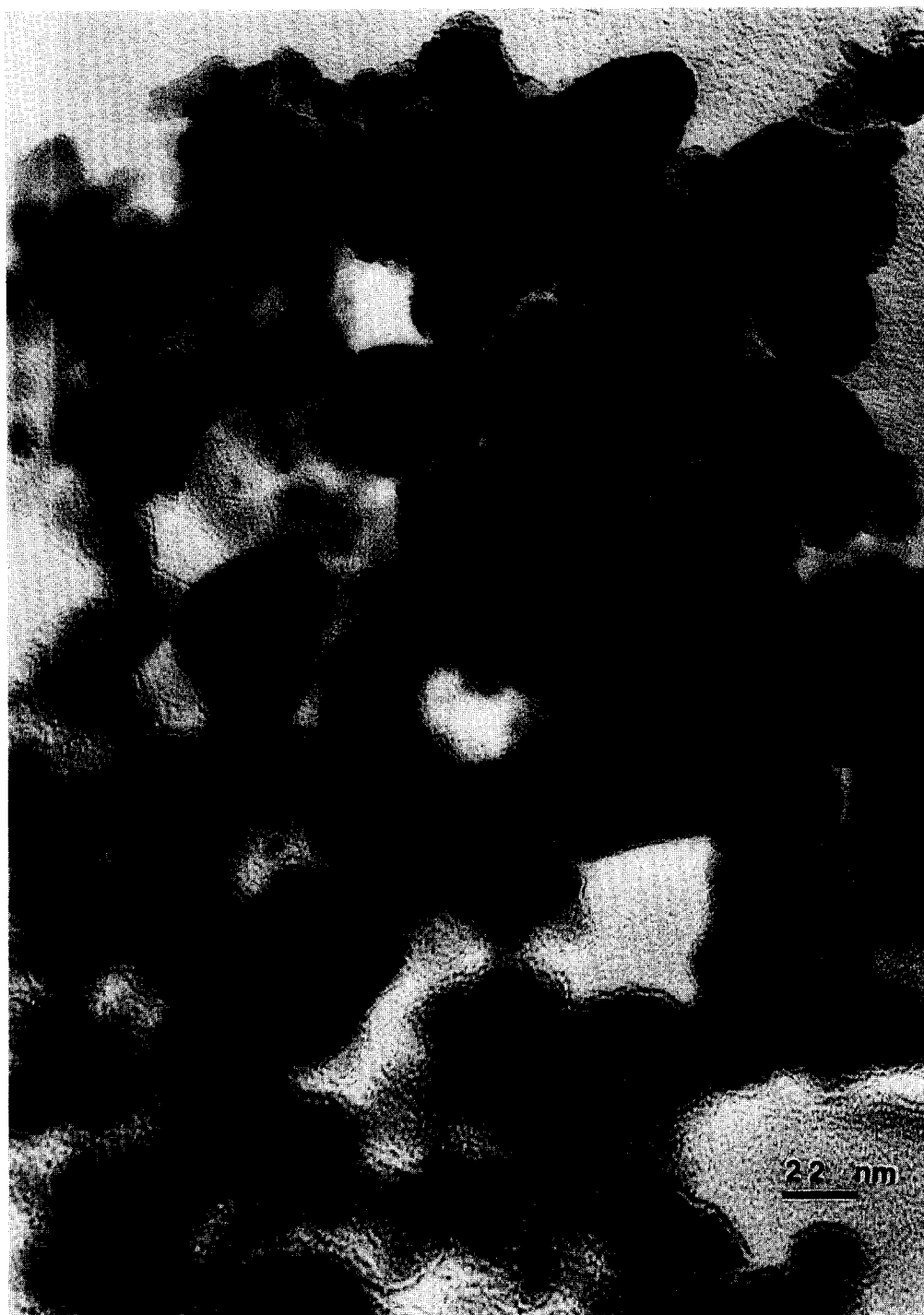
FIG. 12. The bright-field micrograph of CAT-65, prepared by physical admixture technique with 14.2 wt% cobalt and 0.8 wt% Cu.
